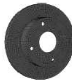
Figure (10) ABAQUS part model & Meshed part
